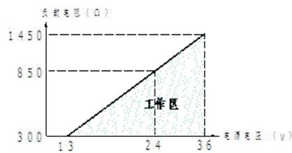
$$\text{最大允许电阻}(\Omega) = 50 \times (\text{电源电压} - 5) - 100$$
